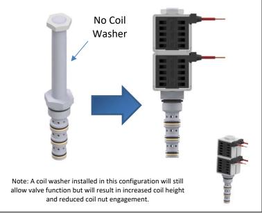
For both coil styles, coils can be installed in "upside-down" or rotated configurations if required.
